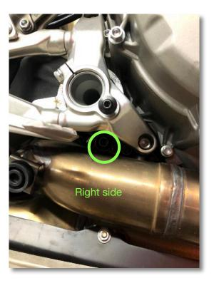
Making safe the area under the bike, loosen the Cat-box front retaining bolts, at the top of the silver bracket at the front of the engine, then release the flange at the rear of the Cat-box downwards, allowing the Cat-box to pivot on the front bolts, then fully remove front bolts.
